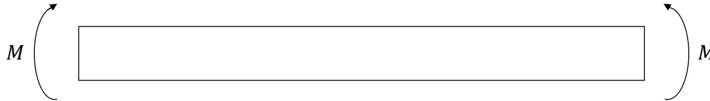
Under these pure bending conditions, the neutral axis (the axis on which there is zero stress) of the beam, also named the elastic line or deflection curve, is a circular arc with radius of curvature,  $R$ , as shown below.
