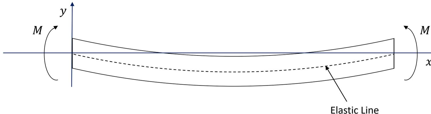
The transverse deflection of the elastic line is given by the co-ordinate,  $y$ , of any position along its length,  $x$
