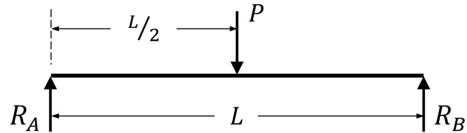
Next, each span between the loading discontinuity is considered separately in order to determine expressions for bending moment,  $M$ .
