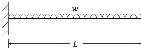
Take origin from right hand side (from free edge – so that reaction force/moment at built-in end are not required) and section the beam as follows:
