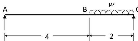
All dimensions in meters,  $w = 10\text{kN/m}$
