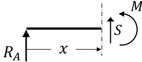
Taking moments about the section position in order to determine an expression for the bending moment,  $M$ , in span 1:
