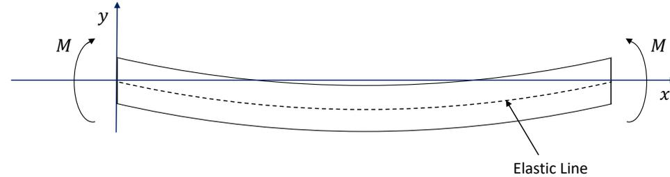
The elastic beam bending equation, which can be used to describe the bending moment,  $M$ , as a function of the radius of curvature,  $R$ , is:  $\frac{\sigma}{y} = \frac{M}{I} = \frac{E}{R}$
