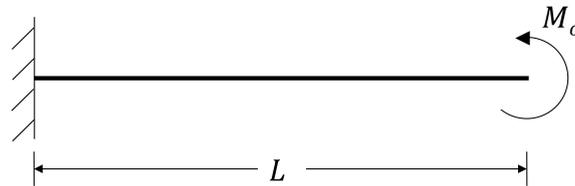
Take origin from right hand side (from free edge – so that reaction force/moment at built-in end are not required) and section the beam as follows:
