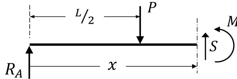
Taking moments about the section position in order to determine an expression for the bending moment,  $M$ , in span 2:
