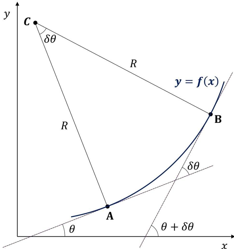
$$\text{Gradient at A: } \left(\frac{dy}{dx}\right)_A = \tan \theta$$
